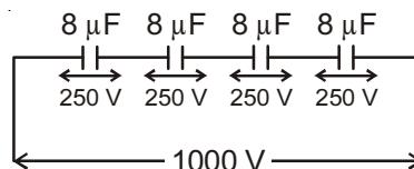
70. In the given circuit diagram when the current reaches steady state in the circuit, the charge on the capacitor of capacitance  $C$  will be :
