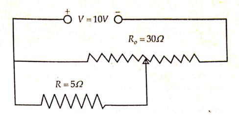
As shown in the *figure* above, a resistance of  $R = 5\Omega$  draws current from a potentiometer of total resistance  $R_o = 30\Omega$ . A voltage V = 10V is supplied to the potentiometer. What is the voltage across R when the sliding contact is in the middle of the potentiometer?
