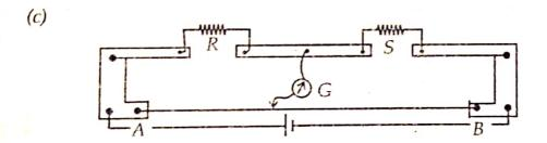
In the meter bridge shown in the above figure, the null point is found at a distance 33.7cm from A and of the wire for particular values of R and S. If a resistance of  $12\Omega$  is connected parallel with S, the null point is found to be at 48.1cm from B end. Determine the value of R and S.
