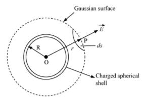
Suppose, we have to calculate the electric field at the point P at a distance r (r > R) from its center. A Gaussian surface is drawn through point P to enclose the charged spherical shell. The Gaussian surface is a spherical shell of radius r and center O.
