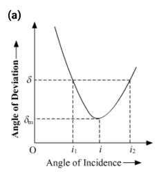
When the angle of incidence and angle of emergence are equal then the angle of deviation of the ray passing through the prism will be minimum.
