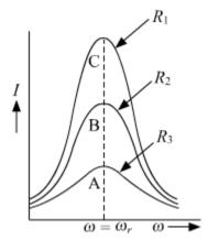
(b) A 2  $\mu$ F capacitor, 100  $\Omega$  resistor, and 8 H inductor are connected in series with an ac source. Find the frequency of the ac source for which the current drawn in the circuit is maximum.
