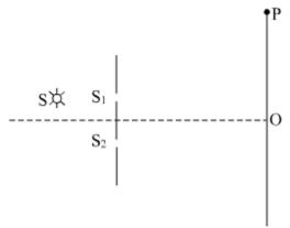
The figure shows a modified Young's double slit experimental set-up. Here  $SS_2 - SS_1 = \lambda/4$ .
