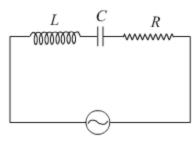
We get maximum current when the LCR Series Circuit is at resonance.
