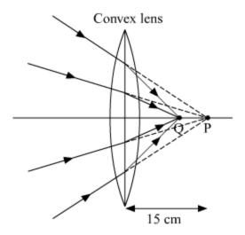
Here the object is a vertical object at P. According to sign convention, Object distance = u = +15 cm Focal length = f = +10 cm
