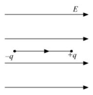
This is stable equilibrium because the potential energy of the dipole here is minimum. As,
