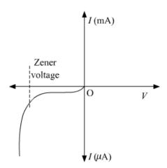
A Zener diode is fabricated by heavily doping both p and n sides of the junction. Because of the heavy doping, a very thin ( $<10^{-6}m$ ) depletion region is formed between p and n sides. Hence the electric of the junction is extremely high ( $\sim 5 \times 10^6 \text{ v/m}$ )
