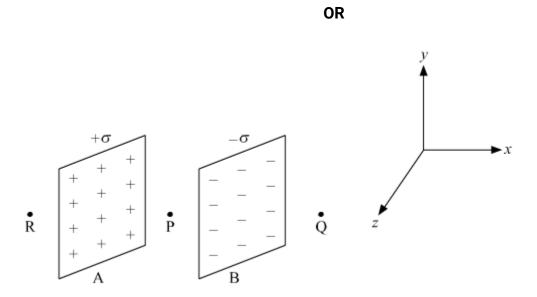
Let *P* is the point between the plates A and B, and *Q* and *R* are the points outside the plates.
