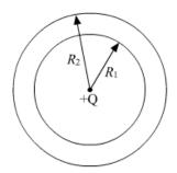
Because of the induction, the inner surface will occupy a negative change '-Q' and the outer surface will occupy a positive charge '+Q'.
