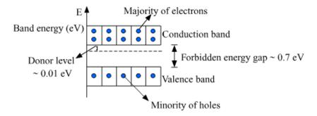
At a temperature of 0 K conduction band of the semiconductor is completely empty and it behaves as an insulator.
