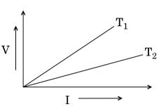
V-I graph for a metallic wire at two different temperatures  $T_1$  and  $T_2$  is as shown in the figure. Which of the two temperatures is higher and why?
