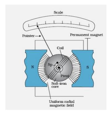
Principle: "Whenever a current carrying coil is placed in magnetic field, it experiences a deflecting torque."
