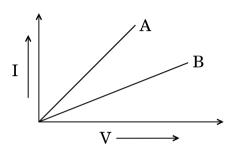
Two metallic resistors are connected first in series and then in parallel across a d.c. supply. Plot of I-V graph is shown for the two cases. Which one represents a parallel combination of the resistors and why?
