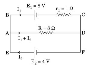
In the electric network shown in the figure, use Kirchhoff's rules to calculate the power consumed by the resistance  $R=8~\Omega$ .
