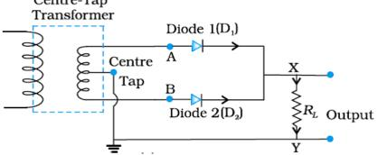
For positive half cycle of input ac, one of the two diodes gets forward biased and conducts and output is obtained across the load  $R_{\rm L}$
