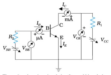
The emitter-base junction, being forward biased, the majority charge carriers (electrons), from the emitter, flow into the base region constituting the emitter current( $I_E$ )
