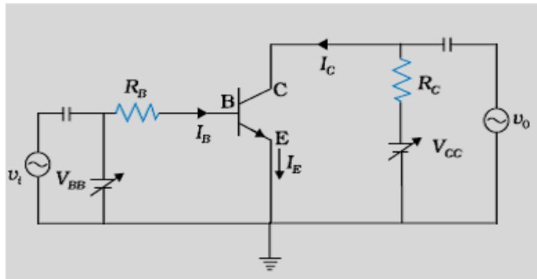
When the sinusoidal voltage is applied on the emitter base circuit, it gets amplified and its phase is reversed.
