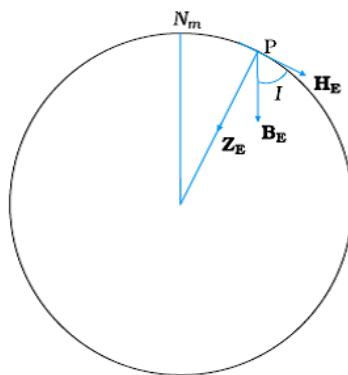
Direction of compass needle is vertical to the earth's surface at poles and is parallel to the earth's surface at equator.
