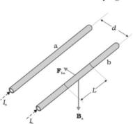
The magnetic field at any point on the wire (b) due to the current in wire (a) is is perpendicular to the plane of two wires and pointing inwards and hence force on it will be towards wire (a). Similarly force on wire (a) will be towards wire (b). Hence two wires carrying currents in same direction attract each other.
