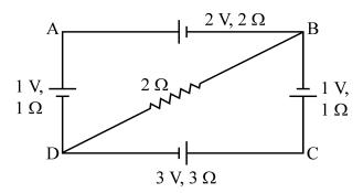
Using Kirchhoff's rules, calculate the potential difference between B and D in the circuit diagram as shown in the figure.
