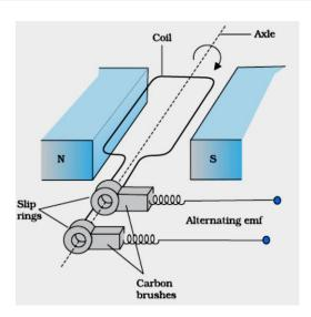
It works on the process of electromagnetic induction, i.e. when a coil rotates continuously in a magnetic field, the effective area of the coil, linked (normally)
