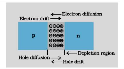
Two processes involved during the formation of p-n junction are diffusion and drift . Due to the concentration gradient, across p and n sides of the junction , holes diffuse from  $p\to n$  , and electrons from  $n\to p$  . This movement of charge carriers leaves behind ionised acceptors on the p-side and donors on the n- side of the junction . This space charge region on either side of the junction , together , is known as depletion region.
