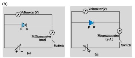
Using the circuit arrangements shown in fig (a) and fig (b), we study the variation of current with applied voltage to obtain the V-I characteristics shown below.
