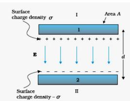
Electric field between the plates of capacitor  $E = \frac{\sigma}{\varepsilon_0} = \frac{Q}{A\varepsilon_0}$
