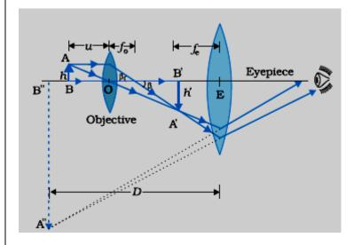
For eyepiece  $m_e = \frac{v_e}{u_e}$   $u_e = \frac{v_e}{m_e} = \frac{-20}{5} cm = -4 cm$
