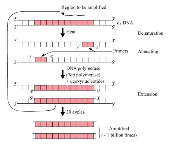
The enzymes used in PCR is Taq polymerase which is obtained from the bacterium *Thermus aquaticus*, which yields DNA polymerase.
