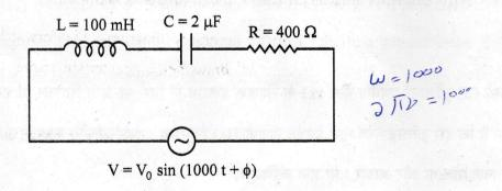
(i) Find the value of the phase difference between the current and the voltage in the series LCR circuit shown below. Which one leads in phase: current or voltage?
