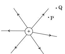
Figure shows the field lines on a positive charge. Is the work done by the field in moving a small positive charge from Q to P positive or negative? Give reason.
