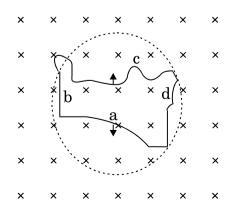
A flexible wire of irregular shape, abcd, as shown in the figure, turns into a circular shape when placed in a region of magnetic field which is directed normal to the plane of the loop away from the reader. Predict the direction of the induced current in the wire.
