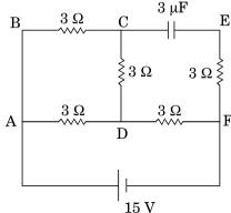
In the circuit shown in the figure, find the total resistance of the circuit and the current in the arm AD.
