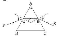
Figure shows a ray of light passing through a prism. If the refracted ray QR is parallel to the base BC, show that (i)  $r_1 = r_2 = A/2$ , (ii) angle of minimum deviation,  $D_m = 2i - A$ .
