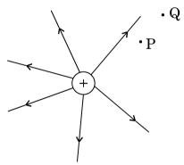
Figure shows the field lines due to a positive point charge. Give the sign of potential energy difference of a small negative charge between the points Q and P.
