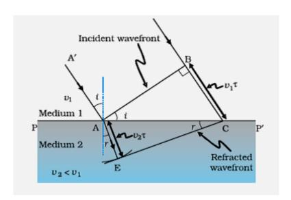
Let t be the time taken by the wavefront to travel the distance BC in rarer medium and AE in the denser medium
