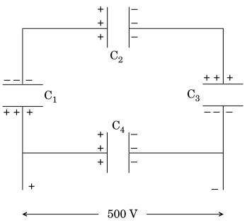
A network of four 10  $\mu F$  capacitors is connected to a 500 V supply as shown in the figure. Determine the
