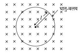
A metallic rod of length 'l' is rotated with a frequency 'v', with one end hinged at the centre and the other end at the circumference of a circular metallic ring, about an axis passing through the centre and perpendicular to the plane of the ring. A constant and uniform magnetic field B parallel to the axis is present everywhere.
