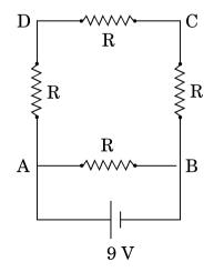
A 16  $\Omega$  resistance wire is bent to form a square. A source of emf 9 V is connected across one of its sides as shown. Calculate the current drawn from the source. Find the potential difference between the ends C and D.
