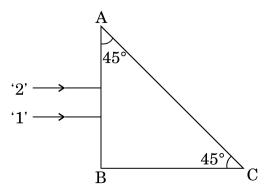
Two monochromatic rays of light are incident normally on the face AB of an isosceles right-angled prism ABC. The refractive indices of the glass prism for the two rays '1' and '2' are respectively 1·3 and 1·5. Trace the path of these rays after entering through the prism.
