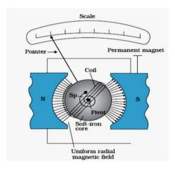
**Principle and working**: A current carrying coil, placed in a uniform magnetic field, (can) experience a torque
