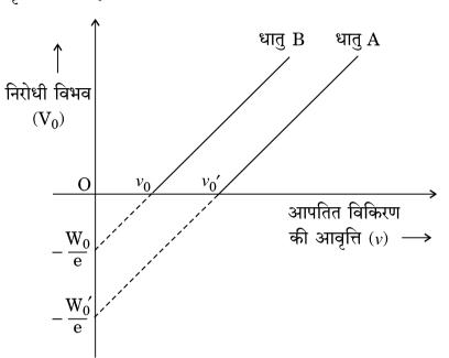
The graph shows variation of stopping potential  $V_0$  versus frequency of incident radiation  $\nu$  for two photosensitive metals A and B. Which of the two metals has higher threshold frequency and why?
