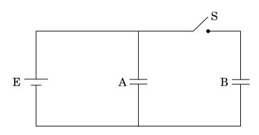
Two identical parallel plate capacitors A and B are connected to a battery of V volts with the switch S closed. The switch is now opened and the free space between the plates of the capacitors is filled with a dielectric of dielectric constant K. Find the ratio of the total electrostatic energy stored in both capacitors before and after the introduction of the dielectric.
