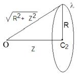
The field at an axial point of a circular loop of radius R and linear charge density  $\lambda$ , is given by
