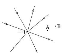
The field lines of a negative point charge are as shown in the figure. Does the kinetic energy of a small negative charge increase or decrease in going from B to A?
