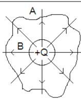
The figure shows two surfaces A and B of different shapes and sizes enclosing a given charge +Q.
